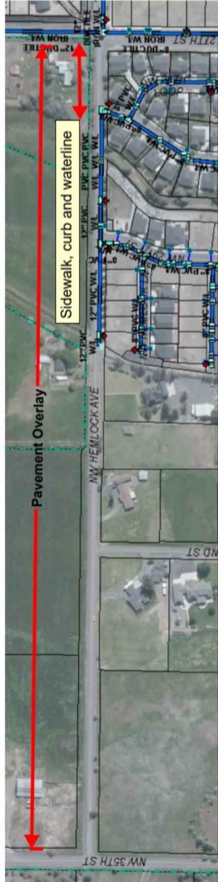
NW Hemlock Ave. from NW 27th to NW 35th: Curb, sidewalk and 12" waterline from NW 27th to NW 28th, pavement overlay from NW 27th to NW 35th.
