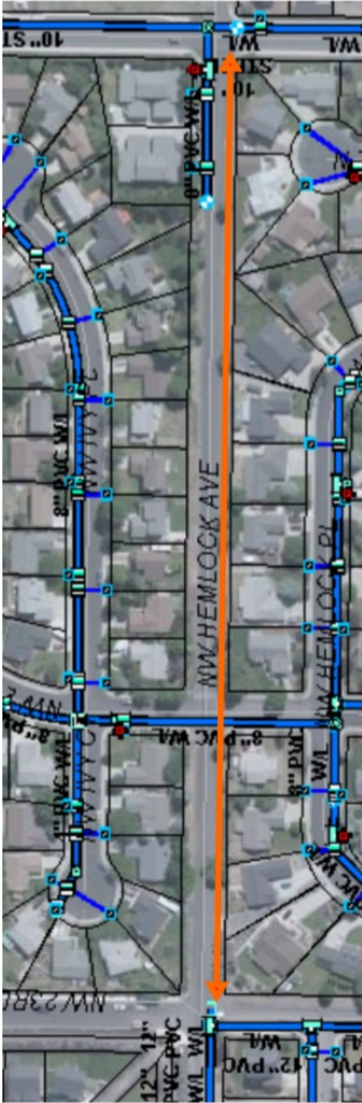
NW Hemlock Ave. from NW 19th to NW 23rd: Complete reconstruction with new curbs, 5' concrete sidewalk on south side, 8' multi-use path on north side, storm drainage, 12" waterline, storm drainage and new pavement and base rock.
